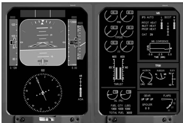
Fig. 5 Glass cockpit display and IMS interface.
